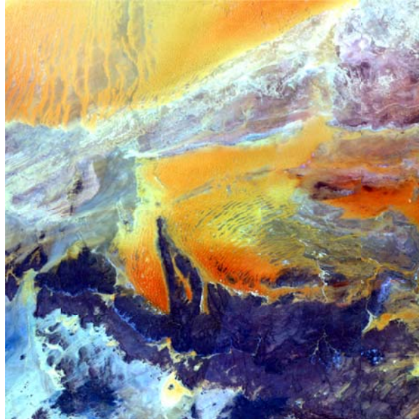
Figure 6-2: Example of CCI-LC SR 7-day composite, at 300m spatial resolution and tile v12h37 - ESACCI-LC-L3-SR-MERIS-300m-P7D-h37v12-20050702-v1.0.nc (RGB with channels 7, 5, 2).
